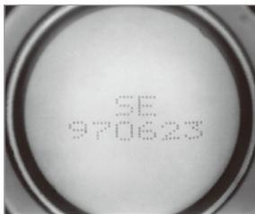
LDM2 Series illuminates light from a wide diffusion area to encompass the entire workpiece. Curved metal surfaces etc. can be illuminated evenly. The bottom of aluminum cans can be illuminated evenly to highlight the letters only.
