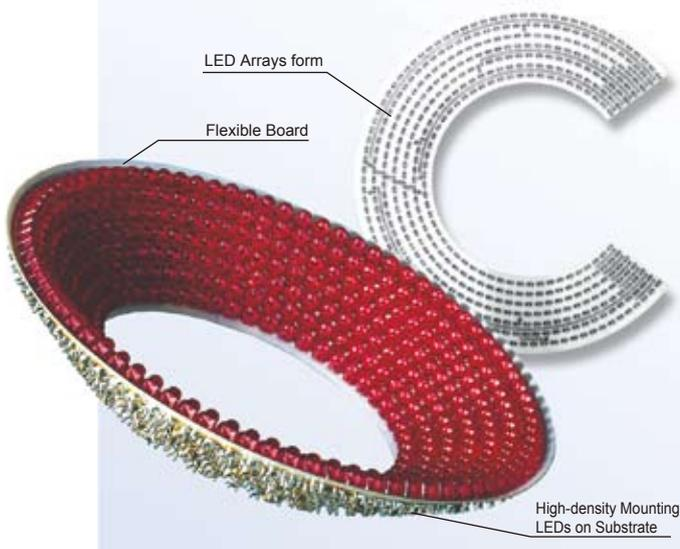
Using a flexible board makes it possible to adjust the outer diameter, inner diameter, illumination angle, and other characteristics to create an illumination system that is ideal for the object being illuminated.
